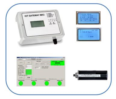
The FMS-00 Fixture Monitoring system uses specially designed Wireless Pressure Transmitters to monitor hydraulic and pneumatic fixtures and transmit to the receiver unit which displays this information and provides both alarm relays and digital communication outputs. The FMS system can operate as a stand-alone system or be fully integrated into any CNC machine with industry standard communications protocols.
