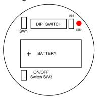
Switches 1, 2, 3 & 4 select the RF Network the IWT will transmit on. The default network for both the IWT transmitter and IWR receiver is network 1.
