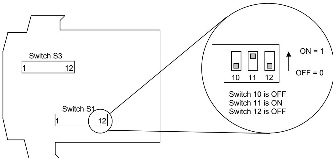
Switch S1 configures the input type and range and switch S3 configures the output type, range and a few additional functions. The switch settings are explained in the next few pages. The diagrams refer to switch positions 0 and 1, with 0 being OFF and 1 being ON. This is illustrated in the picture above.
